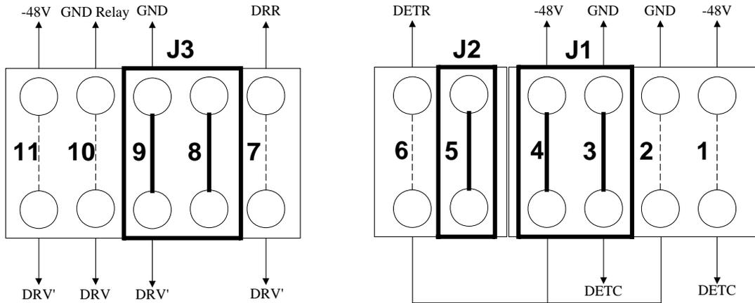
**Figure 11-4. Jumper Switch Configuration**
